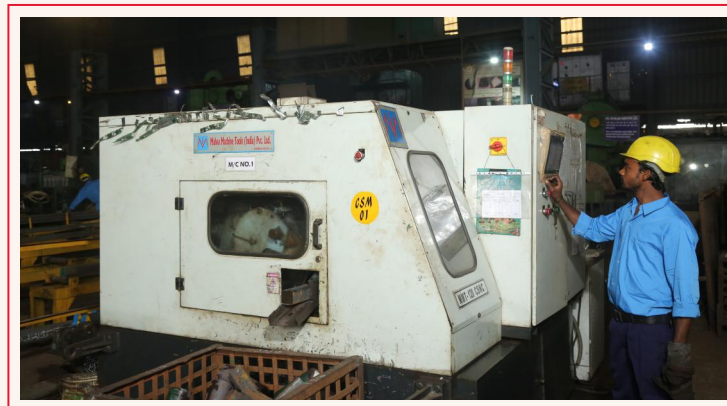
CIRCULAR SAW (FULLY AUTOMATIC) CAPACITY = Ø120 MM | CYCLE TIME = 20 SECOND
